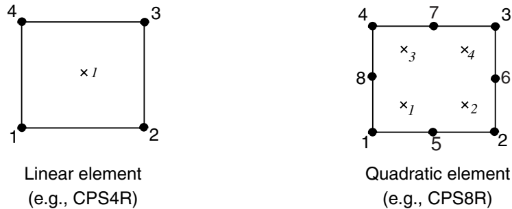
Figure 4-7 Integration points in two-dimensional elements with reduced integration.
